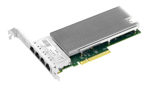
LREG1007PT is a 10G intelligent network adapter based on the chip solution independently developed by Linkreal CO.,Ltd. The product integrates four 10Gigabit Ethernet Medium Access Controller (MAC) and RJ45 port, which not only has the functions of Ethernet MAC and PHY layer, but also can effectively manage network traffic.
