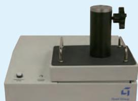
Stud Pull- Coating Adherence Test
