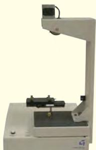
180° Flexible/Rigid Substrate Peel Test
