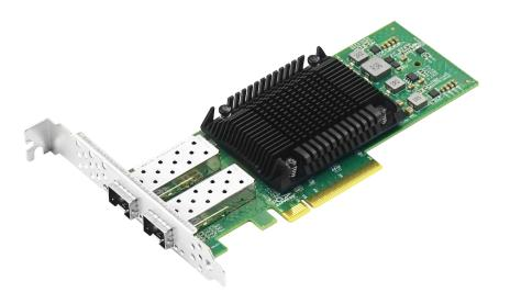
LRES1021PF-2SFP28 is a PCIe v4.0 x8 dual-optical port 25G Ethernet network adapter developed by Linkreal CO.,LTD. on the basis of Intel E810 master program. It is supplemented with hardware accelerated packet processing extended features, while the introduction of application queuing technology, can be optional support for RDMA iWARP and RoCEv2 function, the adapter can be simultaneously backward compatible with PCIe v3.0 & v2.0.
